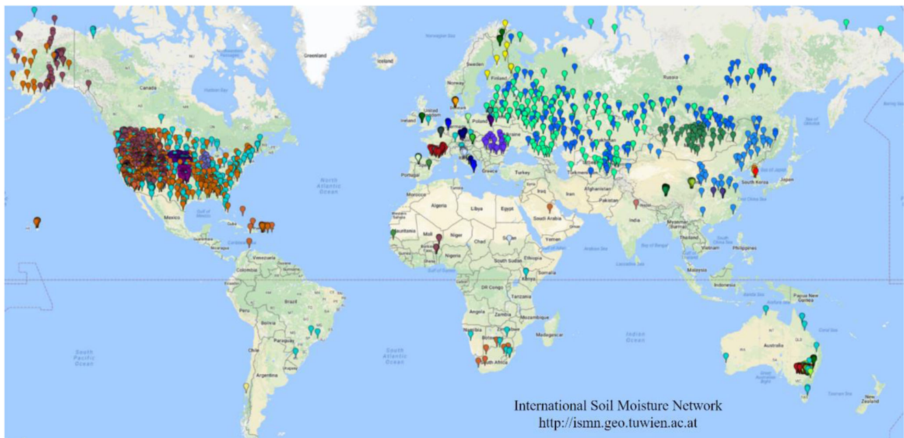
Fig. 2 Distribution of ground stations for measuring soil moisture from ISMN consisting of 2439 ground stations from 59 networks (April 2019)
